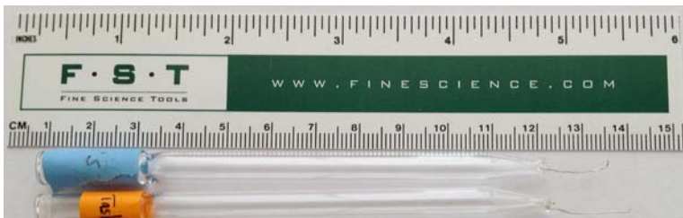
Figure 1. Shown are platinum-wire worm picks used to move C. elegans . These simple worm picks can be made in the lab.
